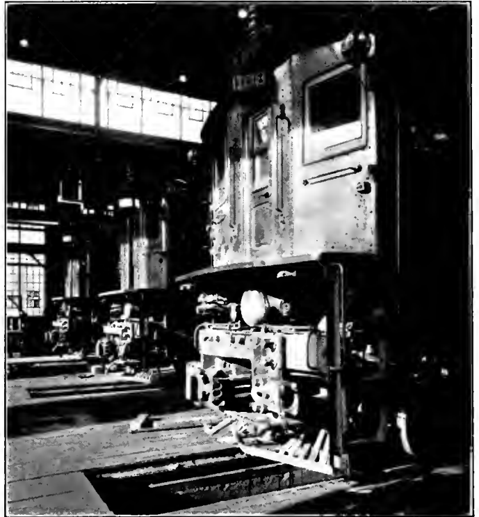
Interior View of Virginian Railway Shop Showing Drop Pits
